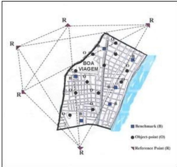
Figure 5 : GPS monitoring network
